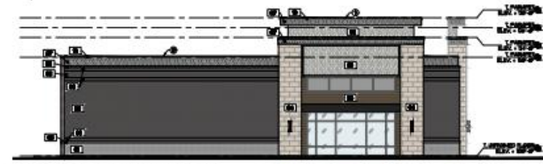
④ WEST ELEVATION TOTAL HEIGHT OF - 14'6" IF TOTAL HEIGHT OF - 12'6" IF SCALE 1/8" = 1'-0"
