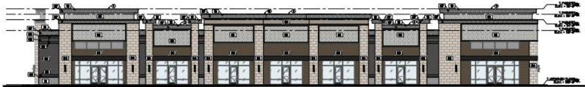
① SOUTH ELEVATION TOTAL HEIGHT OF - 14'6" IF TOTAL HEIGHT OF - 12'6" IF SCALE 1/8" = 1'-0"
