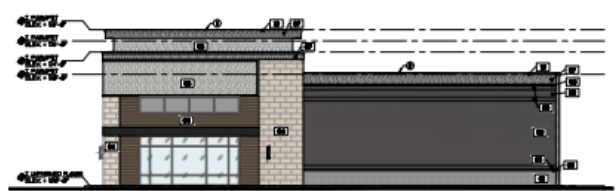
③ EAST ELEVATION WALL THICKNESS - 12" OF SCALE 1/4" = 1'-0"
